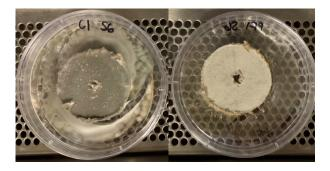
The control sample is on the left and the sample treated with the Mold Guard Pharmaceutical formula is on the right. Photos were taken 20 days after inoculation with penicillium chrysogenum. The control sample was completely covered in fungi within the first few days. The sample treated with Mold Guard showed 0 growth after 20 days.
