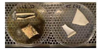
The control sample is on the left and the sample treated with the Mold Guard food formula is on the right. The picture was taken 20 days after inoculation with chaetomium globosum. The control sample was completely covered in fungi within the first few days. The sample treated with the Mold Guard food formula showed 0 growth after 20 days.
